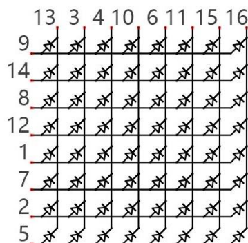
Connection mode of Common Anode
